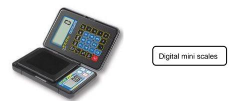
**Digital scales** (sometimes sold as 'electronic balances') can be expensive, especially if they are precise enough for artefact recording. Ideally we would like measurements to one-hundredth of a gram (two decimal places). Electronic kitchen scales that measure to the nearest gram can be used if there is nothing else available.
