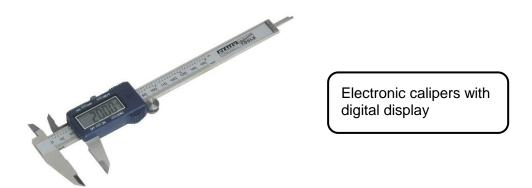
**Calipers** can be digital or analogue. Digital calipers measure to one-hundredth of a millimetre (two decimal places), but we only need a precision of one-tenth of a millimetre (one decimal place). If you only have a ruler and can only take a measurement to the nearest millimetre (or half a millimetre) that is acceptable.
