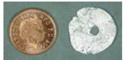
Right: Damage to silver short-cross penny through over-cleaning with sodium hydroxide (caustic soda)
